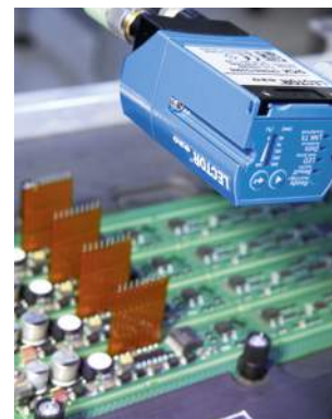
Quality assurance of freshly applied direct marked codes on PCBs
