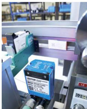
Reading and verifying Data Matrix serialization codes on pharmaceutical packages
