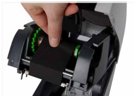
Insert the empty core at the top and twist until the empty core has been completely wrapped.
