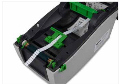
Loosely fit guide rails to the material.
